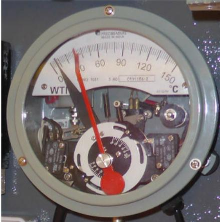
Winding Temperature gauge (WT) - *Figure 7.*
