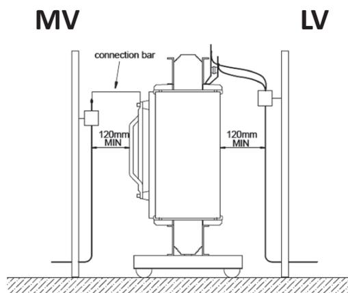
Figure 14 - Cables coming from the bottom.
