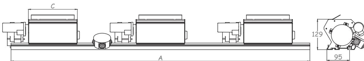
Figure 11 – Tangential ventilation bar (front view)
