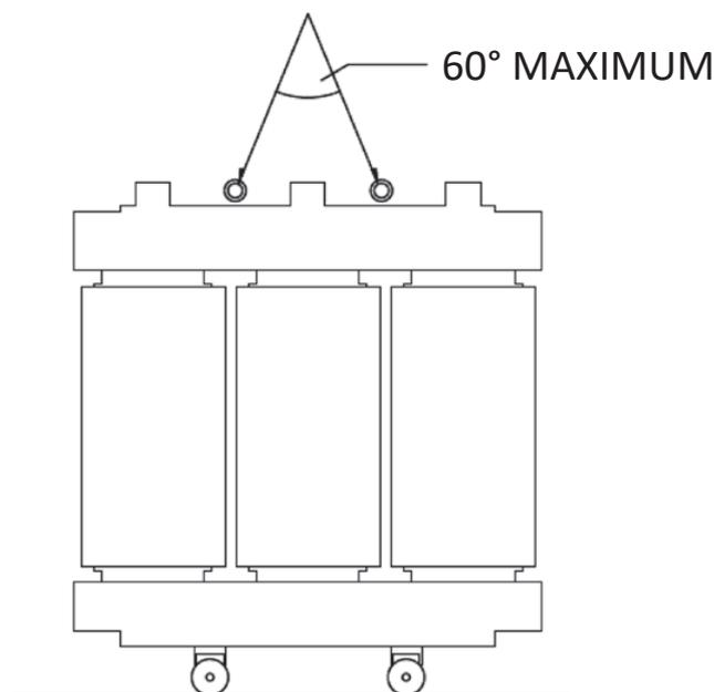
Figure 4 – Handling with overhead-travelling crane
