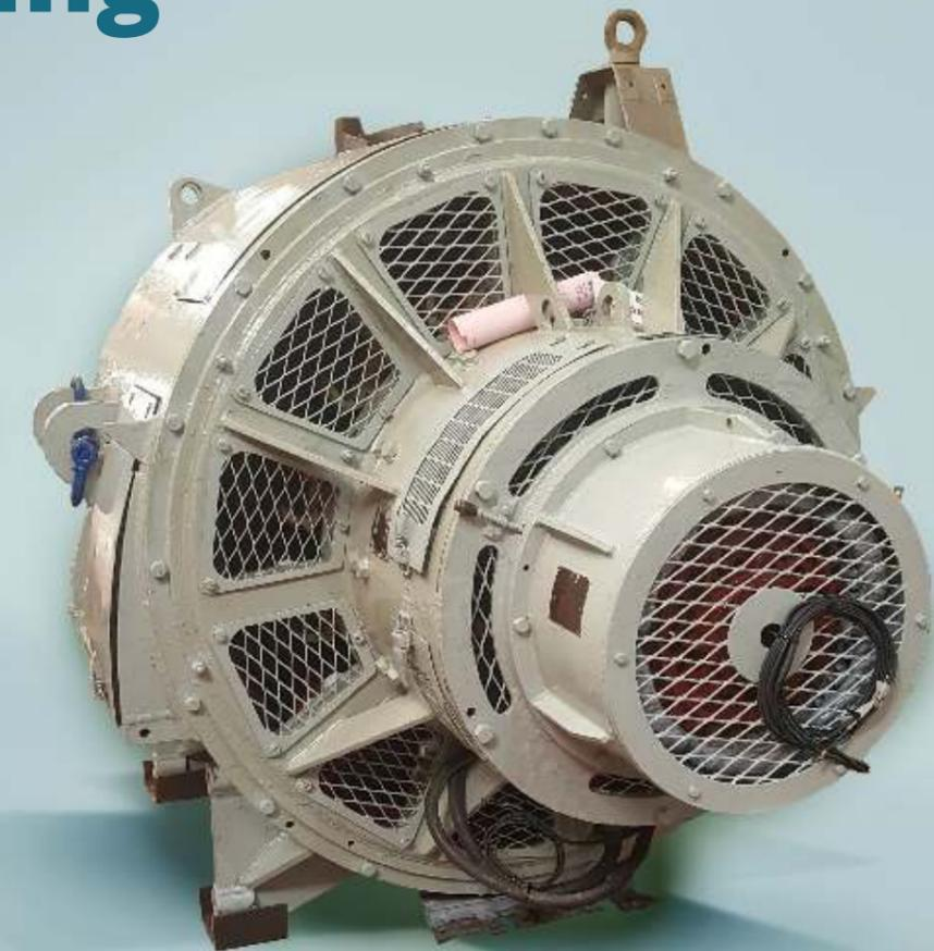
(Right) 2000 HP Stator from a Mather & Platt Electric Motor used to drive a Hydrogen Pump.
